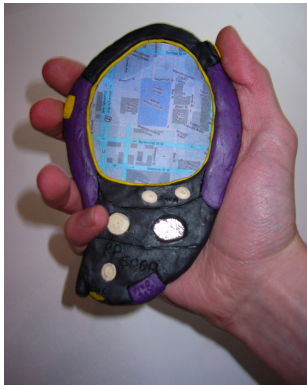
Figure 2. This plasticine prototype enabled us to accurately visualize the size of the device, as well as locations of buttons and control pad.
