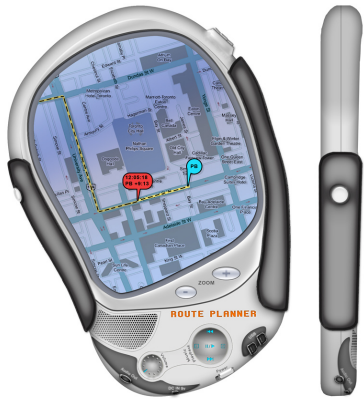
Figure 1. A fully realized visual rendering of the RP. A right-handed version of the device is shown, although it can be reversed to suit the needs of left-handed users.
